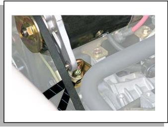
Fig. 24 Adjust Belt Tension
