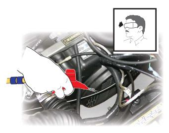
Fig. 27 Cleaning Cooling System with Air
