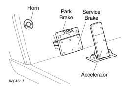
Fig. 5 Accelerator, Brake and Horn Controls
