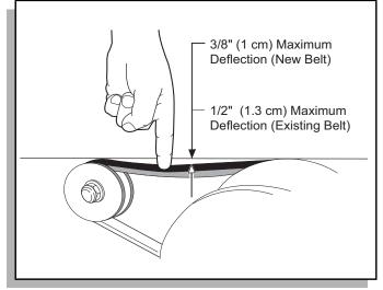
Fig. 23 Check Belt Tension Manually
