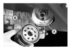
Fig. 19 Inspect Oil Filter
