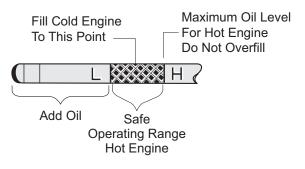
Fig. 15 Check Oil Level on Dipstick
