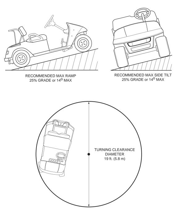
Fig. 36 Vehicle Incline Specifications and Turning Clearance Diameter
