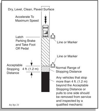
Fig. 26 Typical Brake Performance Test
