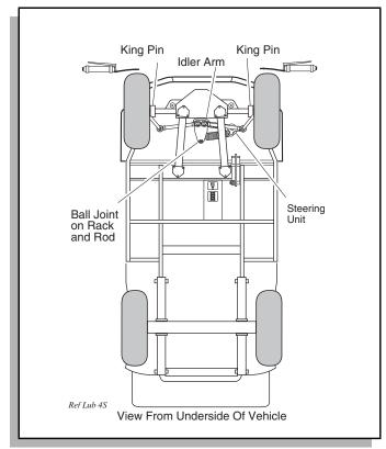
Fig. 30 Lubrication Points
