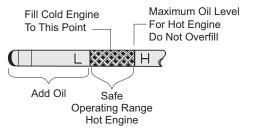
Fig. 6 Check Oil Level on Dipstick
