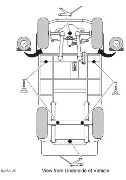
Fig. 9 Lifting the Vehicle
