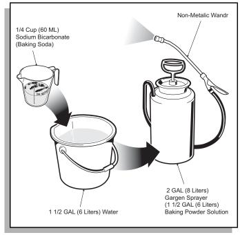
Fig. 25 Preparing Acid Neutralizing Solution
