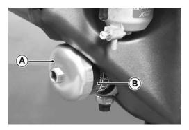
Fig. 18 Remove Oil Filter
