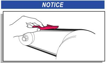
Fig. 22 Check Belt Tension with Gauge
